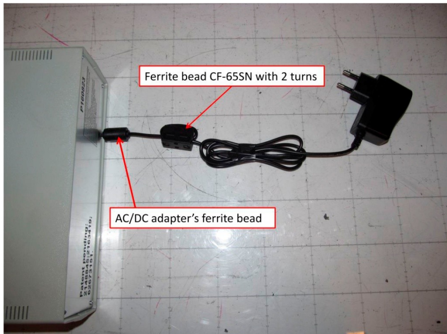
Ferrite bead placed outside the second sample on the AC/DC adapter's power cable
