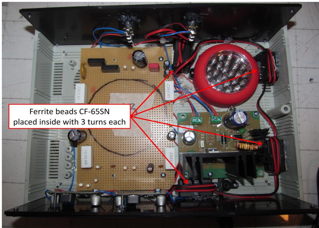
Ferrite beads placed inside the second sample
