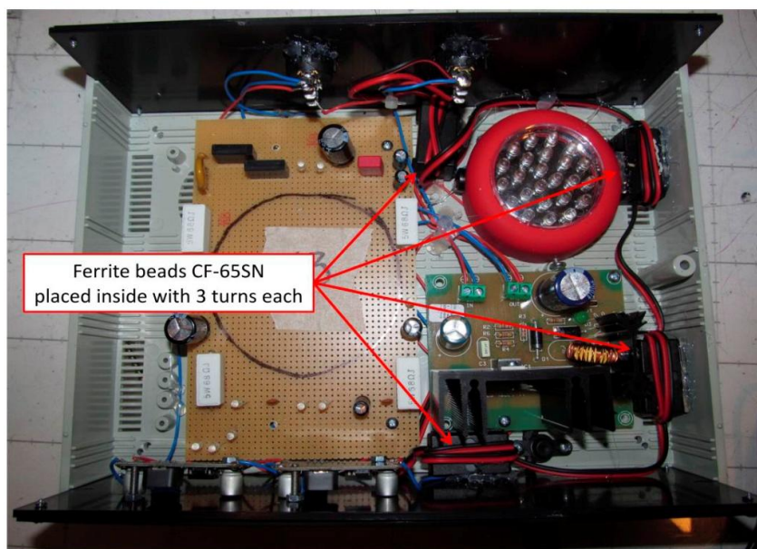
Ferrite beads placed inside the second sample
