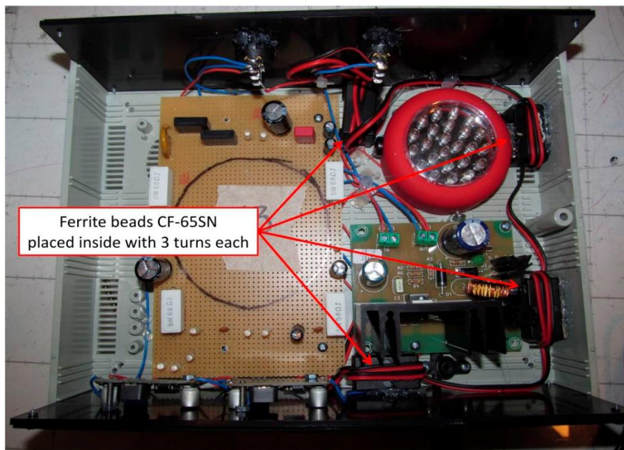
Ferrite beads placed inside the second sample
