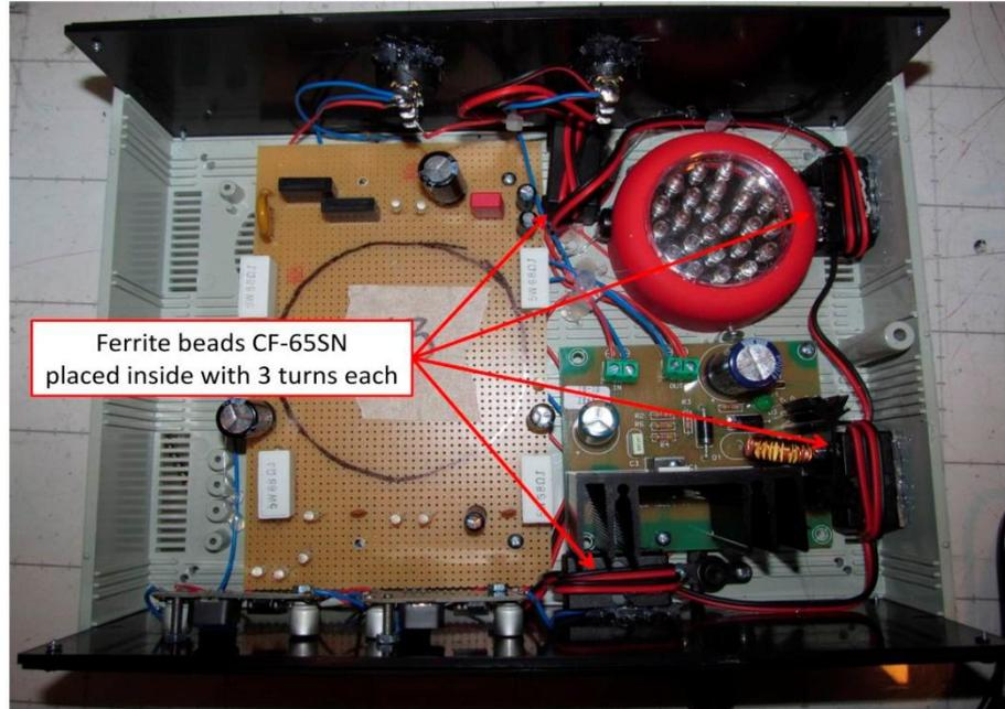
Ferrite beads placed inside the second sample
