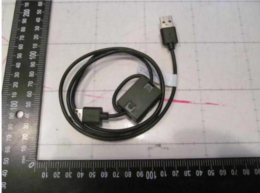
EUT, USB power supply cable (95 cm length)
